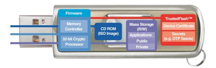
TrustedSignins is based on SanDisk's TrustedFlash technology. Every TrustedFlash device contains a unique readable electronic serial number, a device certificate, and an unknown random encryption key. A custom controller partitions memory and manages access from the host PC. A 32-bit cryptographic co-processor automatically encrypts and decrypts all data written to and read from the device, protecting against information disclosure even if the components are directly targeted.
